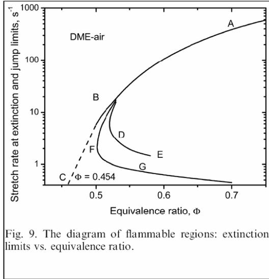
Fig. 9. The diagram of flammable regions: extinction limits vs. equivalence ratio.
